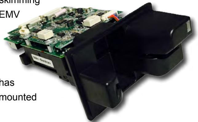
If such device is detected, the ATM will go out of service, and report the incident to its remote monitoring system. Along with detection, when a card is inserted into the card reader, jamming signals interfere with the ability of the skimmer to read the mag-stripe. Moreover, the card reader encrypts the mag-stripe data to defeat an eavesdropping attack inside the ATM.
