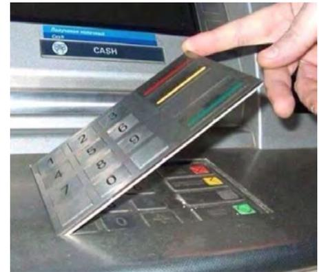
*ATM PIN capture overlay device pulled back to reveal the legitimate PIN entry pad.*
